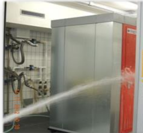
...Water jet test ...
